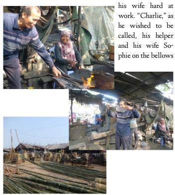
were busy forging iron into ax heads and meat cleavers. The axes are used to cut down large 30 foot bamboo stalks that
