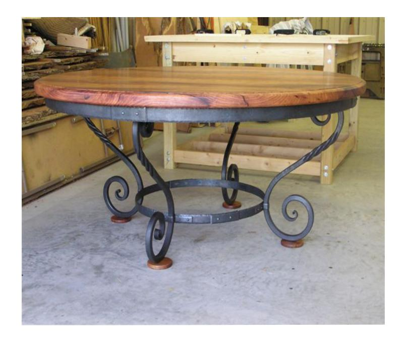
This is a 66 inch table, the top is 2 inches thick. Legs are 1 inch. Hope you like the lap joints and rivets. I should have another one that will be 60 inches by the time of the demo. The trade item is a center punch for indexing work that will be hot worked (blacksmith center punch). See you all then.
