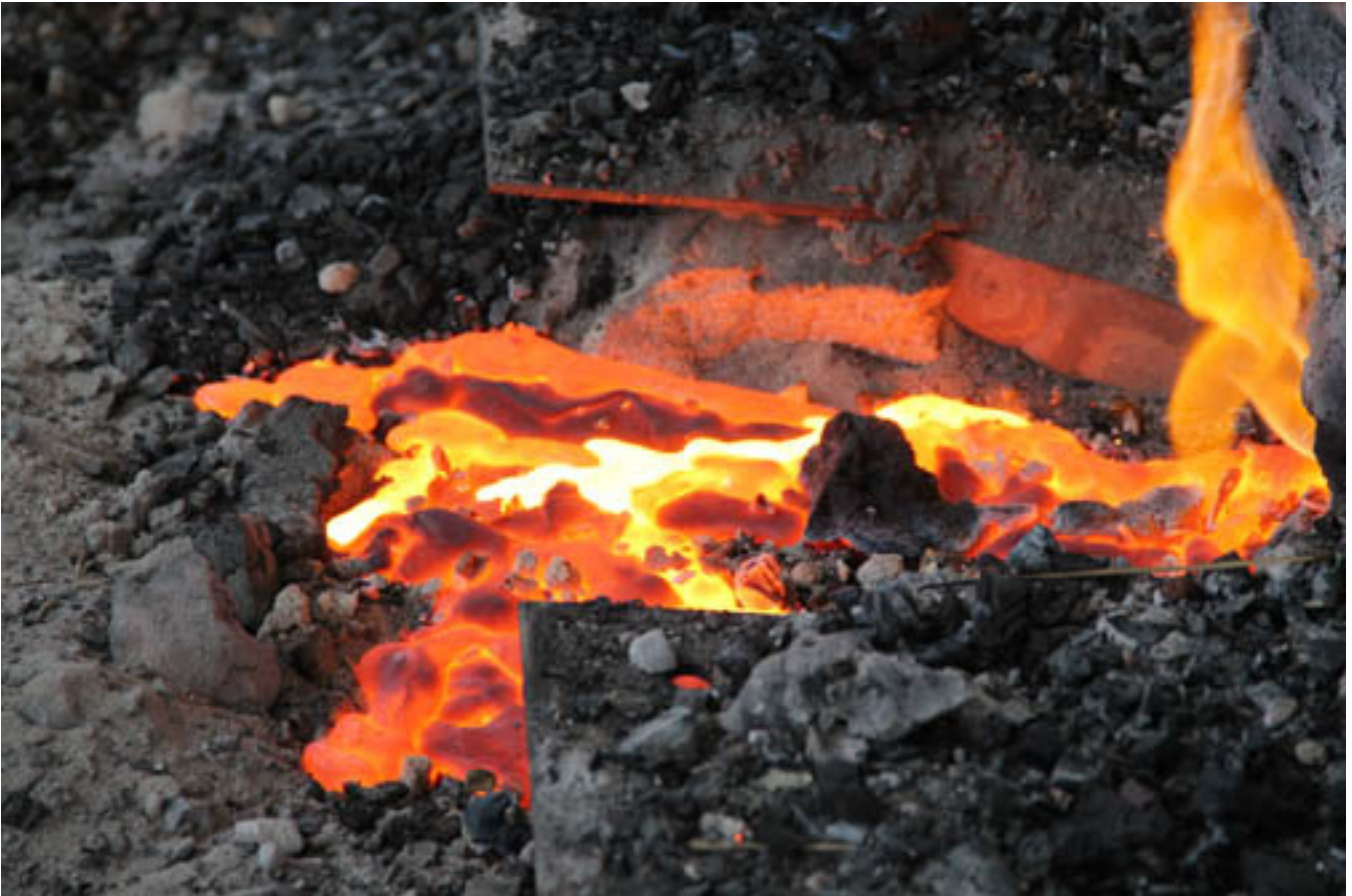
ABOVE: slag drains from the furnace. photos by Vince Herod
