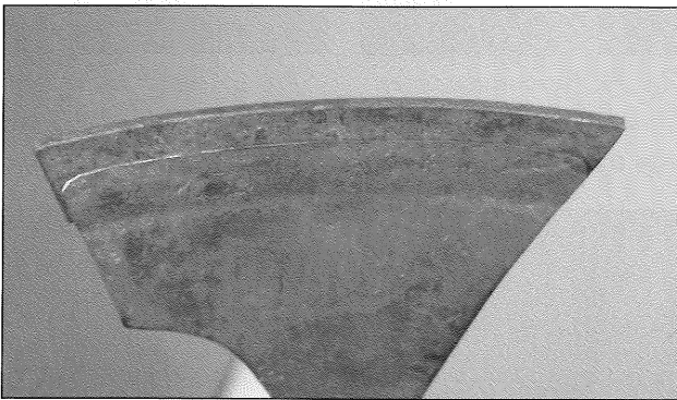
Fig. 42. Steel and blade shown before forge welding. The blade protrudes out from the sides by \frac{1}{16} " to help prevent cold shuts from being formed during welding
