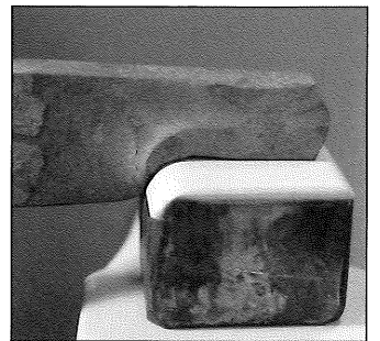
Fig 7. An anvil block with a \frac{1}{2} " radius edge was used to protect the curved transition
