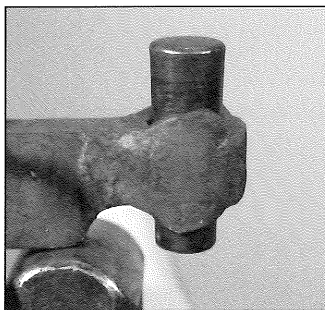
Fig 27. A short mandrel was used to protect the eye as the throat was drawn out
