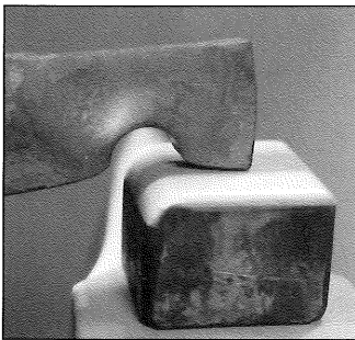
Fig 6. The short side of the fullered groove is drawn down to 1-inch square
