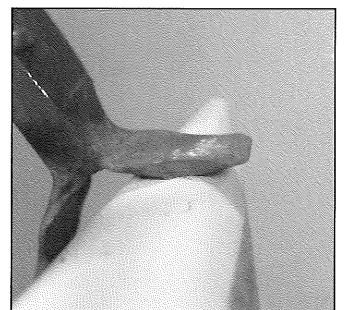
Fig 21. Roll the eye over the bick or a suitable mandrel
