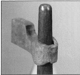
Fig 24. The eye is fitted to contact the mandrel at the weld site
