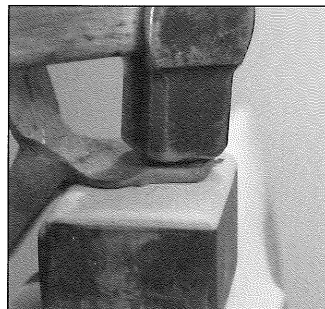
Fig 18. Draw the outside of the eye down to form a tapered scarf
