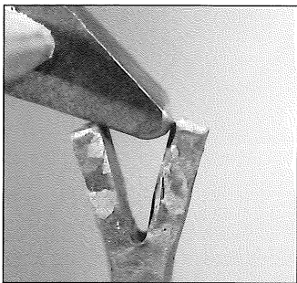
Fig 12. Open out the sides to help prevent cold shuts from being formed
