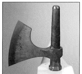
Fig 23. The axe will fit onto the tapered mandrel with the top held downwards
