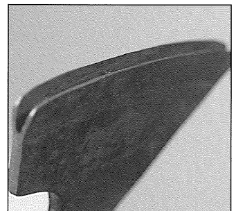
Fig. 38. The finished cut ready to be steeled
