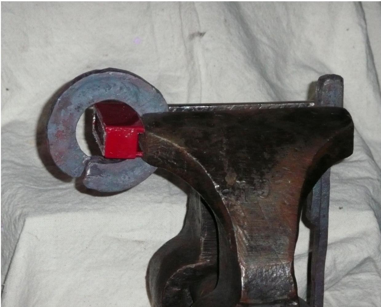
The wedge is made from a 5" piece of  $\frac{3}{4}$ " mild steel, forged into an 8" long wedge. The wedge tapers gradually to about  $\frac{1}{16}$ " thick. When bending the wedge into a circle, it helps to bend the thick side first. The magnet is about 2" long and can be purchased at Harbor Freight.
