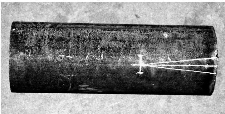
Figure 3 and 4: Pipe marked ready to cut
