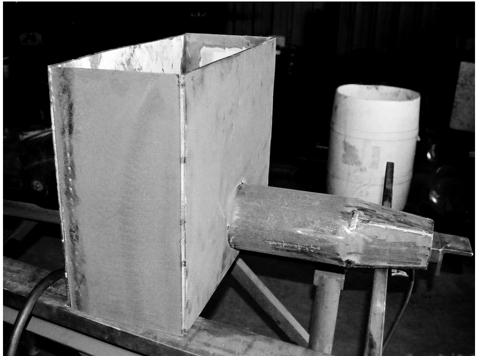
Figure 7: Bosh and water jacket
