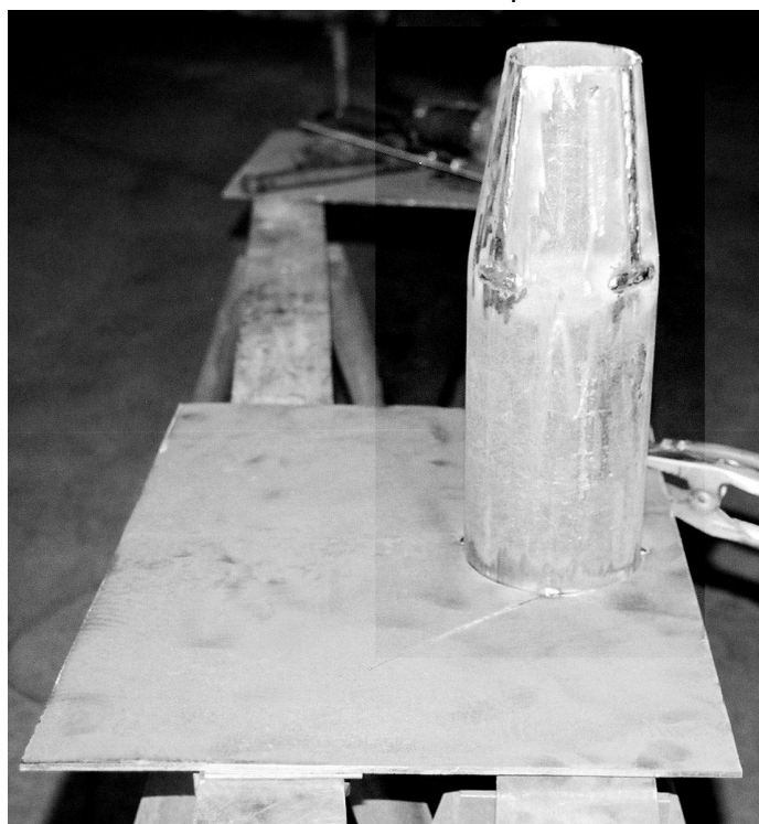
Figure 6: Water jacket tacked in place
