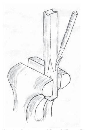
Cutting the horns with "head" clamped in the vise. Keep the hot cut point into the bar; it wants to go vertical on it own.
