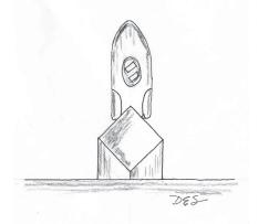
Looking from the side of the anvil setting the eye is done "on the diamond". The second eye will be done by turning the stock 90 degrees and also on the diamond.
