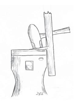
Drawing out the horns – work with square cross section – first one side then rotate 90 degrees and work the other.
