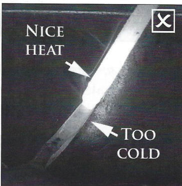
Both parts look wet, but one side is too cold to weld
