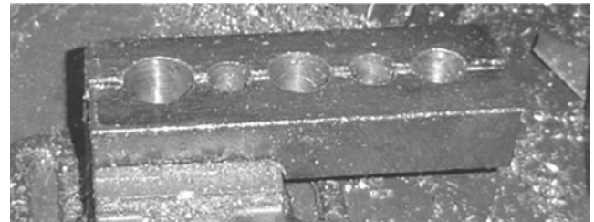
The bundle is drilled and chamfered
