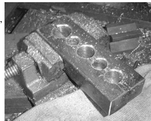
The bundle is drilled and chamfered
