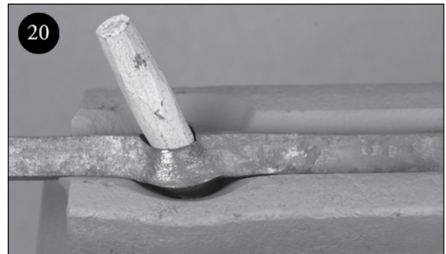
Here, a square bar that has been punched across the corners is being drifted in a bolster
