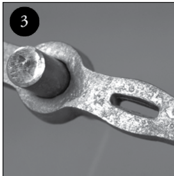
A slot-punched hole drifted to round
