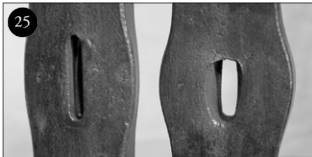
These two photographs show a slot punched hole being upset prior to being drifted. The bar on the left of each photograph shows the initial slot-punched hole for comparison. Upsetting the bar leaves you with more material surrounding the hole
