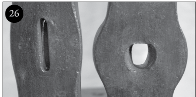
These two photographs show a slot punched hole being upset prior to being drifted. The bar on the left of each photograph shows the initial slot-punched hole for comparison. Upsetting the bar leaves you with more material surrounding the hole
